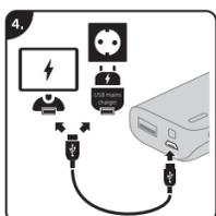
4. Recharge the powerbank via the micro USB port. Connect the charging cable to a bus-powered USB port of your computer or a separate power supply.
