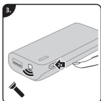
3. Press the function key twice to turn on the LED torch. Press the key twice again, to turn it off.
