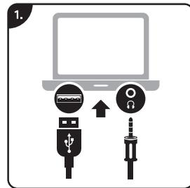
1. Connect the speaker system to your computer via the 3.5mm jack plug and USB cable. Turn on the speaker system. It will be detected automatically and is ready to use.
