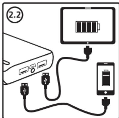
**Note:** The maximum output of the powerbank is limited to 3.0A. If your connected devices require a higher output, the powerbank does not start to charge. Please charge your devices individually then.
